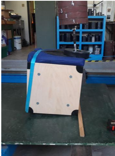
Figure 10. The stability test with gliders
