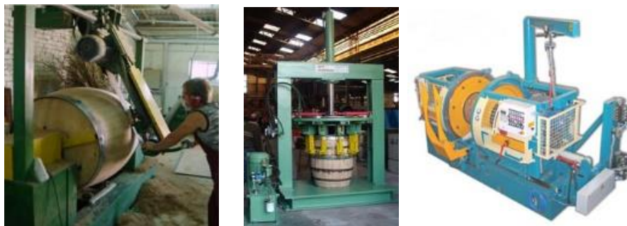
Figure 8. Barrel sanding machine (left), the hooper and heavy-duty barrel crozer (right) (source: Web 7/left; Web 5/middle; Web 6/right)
