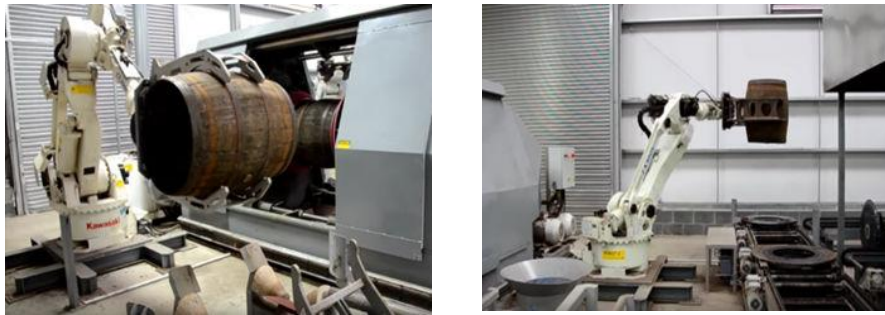
Figure 3. Robots used for barrel manipulation (source: Web 2)
