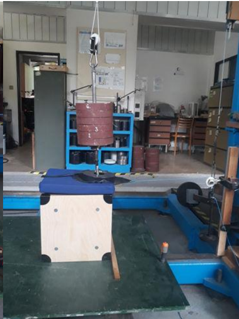
Figure 11. The stability test without gliders
