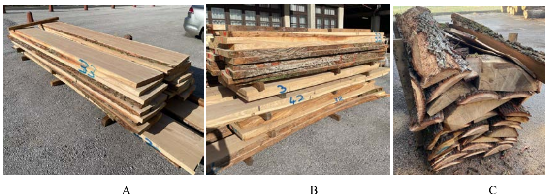
Figure 5. A - Edged and half edged sawn boards, B – Un-edged and half edged sawn boards C - Large wood waste
