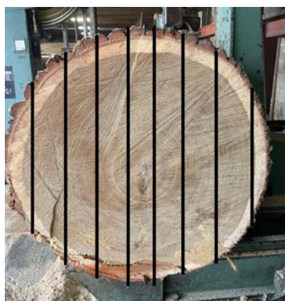
Figure.2. Sawing pattern for live sawing method.
