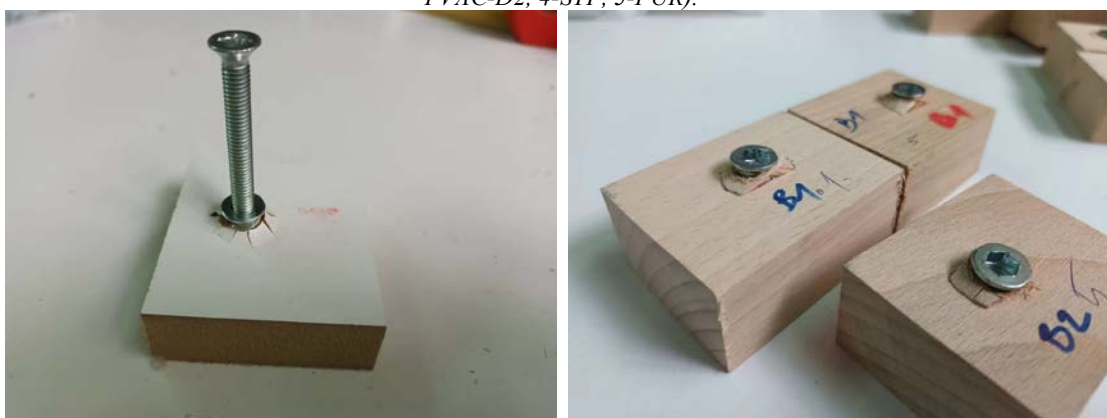
Figure 5. Typical failure mode of MDF and beech specimens.
