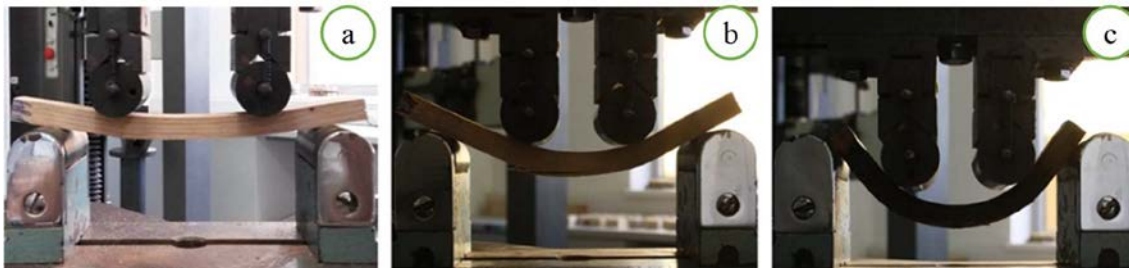
Figure 2. Typical bending test specimens in the material testing machine at the moment of failure: untreated (a), compressed along the grain and fixated for 1 minute (b), and compressed and fixated for a long time, which did not break during the bending test (c).
