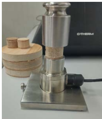
Figure 2. Measurement performed with C-Therm, hot disk method. In background, samples of 30 and 100 mm diameter can be seen with hardwood and sapwood on surfaces
