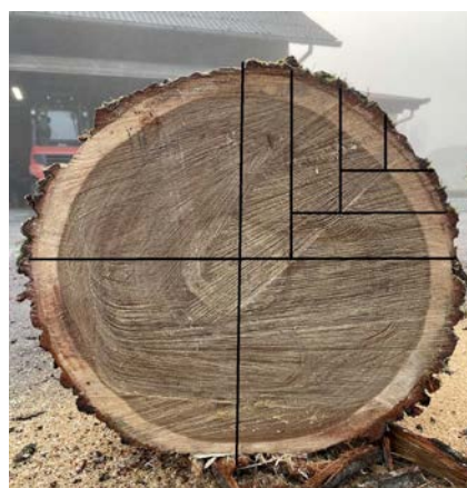
Figure.3. Sawing pattern Slavonian sawing method.
