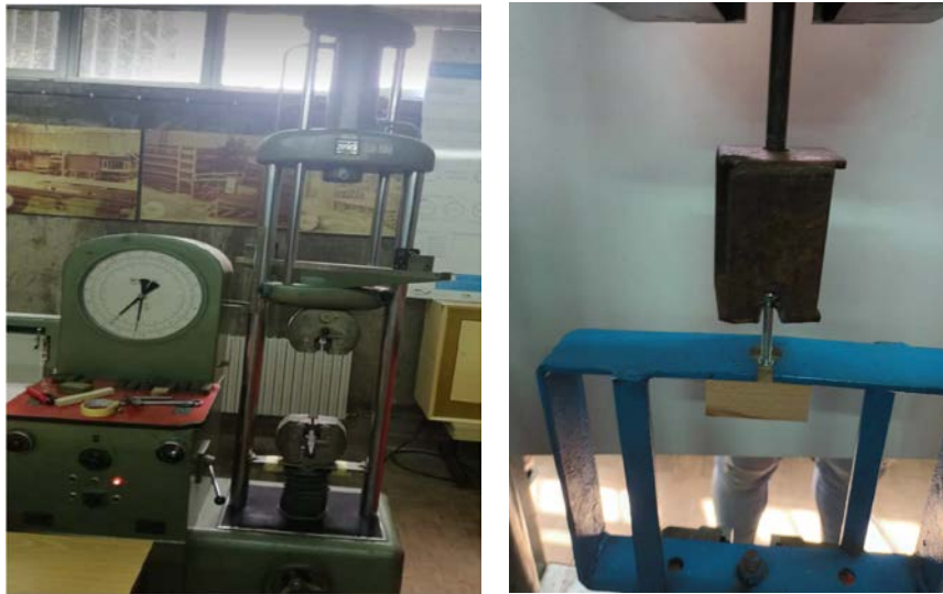
Figure 3. ZWICK testing machine, and testing procedure.
