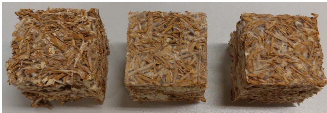
Figure 1. Produced specimens of MBB, from the left P. ostreatus, G. lingzhi and G. lucidum
