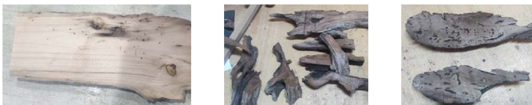
Figure 3. The shapes and wood defects of the driftwood cut samples.
