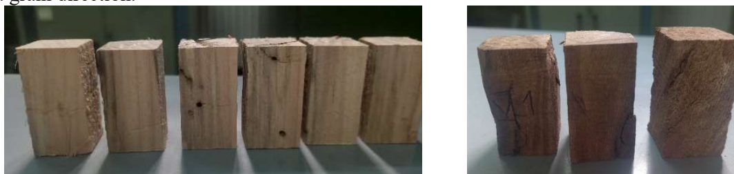
Figure 7. Wood specimen failures of compressive strength parallel to grain testing: poplar with wood defects (left), sycamore wood (right).
